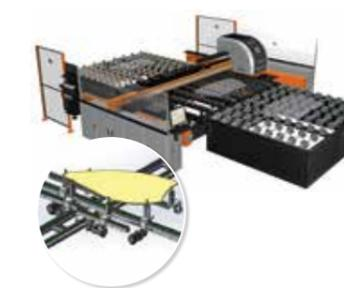
It includes an inline automatic indexing system that is able to automatically index and register shaped glasses, with no manual operation required.
